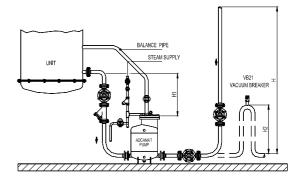
Condensate recovery - open system. The pump removes high temperature condensate without cavitation problems.
